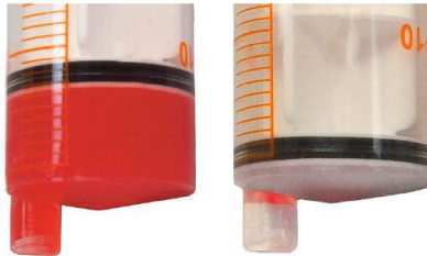
Figure 4. Medication drawn from a cup but administered into an ENFit device can lead to over-delivery of medication. The volume of medication in the tip of the syringe differs before and after administration. The full dose plus the extra in the dead space was administered.
